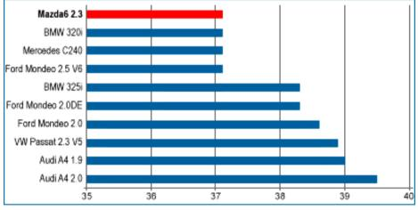
Braking distance (m) from 100 km/h to zero
