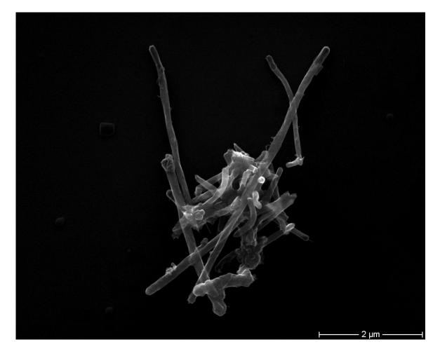
Figure 6: Rigid carbon nanotubes (photograph: BAuA/Fox).
