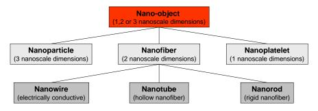
Figure 8: Order of nanomaterials by means of their shape through the introduction of the term nanoobject in accordance with the proposal in DIN ISO/TS 27687:2010-02 "Nanotechnologies - Terminology and definitions for nano-objects – Nanoparticle, nanofibre and nanoplate".
