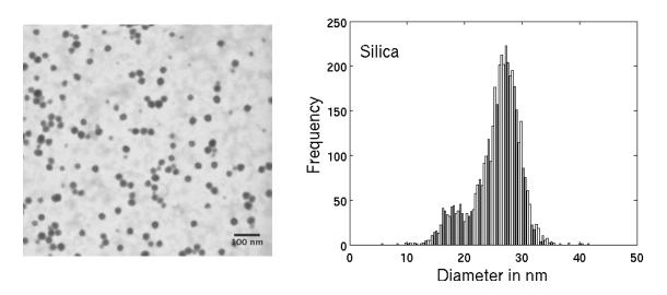
Figure 3: SEM image in transmission from a test specimen of nanoscale silicon oxide particles (left) and the results of a histogram analysis of the diameter distribution of 4400 particles (right), average diameter:  $25.2 \text{ nm} \pm 1.1 \text{ nm}$  (photograph: PTB).
