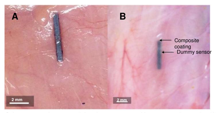
Subcutaneous tissue containing dummy sensor without composite coating (A) and composite coated dummy sensor (B).
