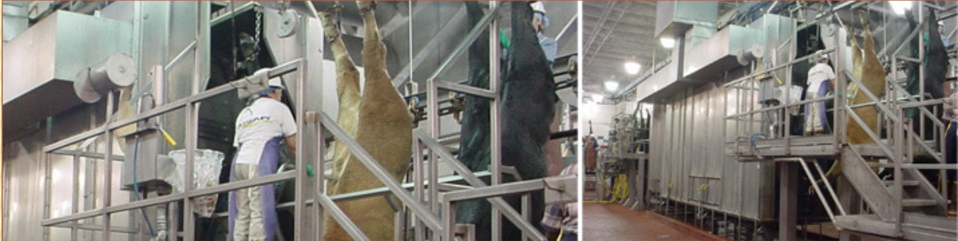
Cargill's system includes a water and sodium hydroxide mix to release contaminants, followed by a high-pressure rinse and lactic acid application.
