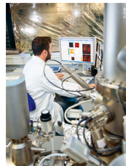
Silver can be detected on coated textile fibres using time-of-flight mass spectrometry.
