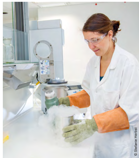
The preparation of the cheese samples for testing involves homogenisation with liquid nitrogen.
