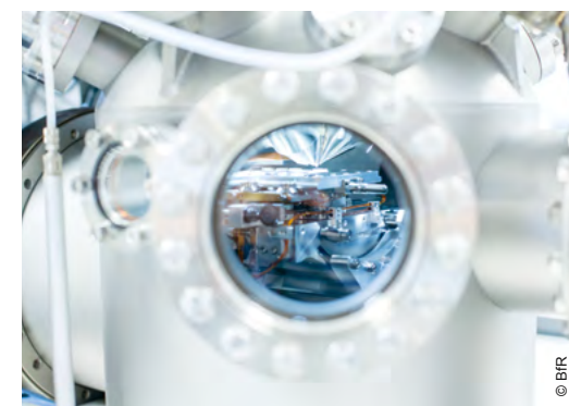
Silver can be detected on coated textile fibres using time-of-flight mass spectrometry.
